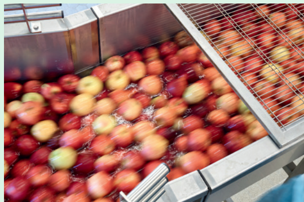
Water is the main means of transport for the apples processed at VOG Products.
